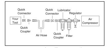
Figure 2. Installing your tool.
